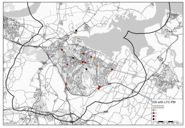
Figure 6-43: DS with LTC, Junction Level of Service, PM Peak
