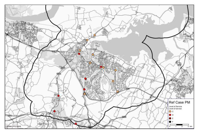
Figure 6-11: RC, Junction Level of Service, PM Peak
